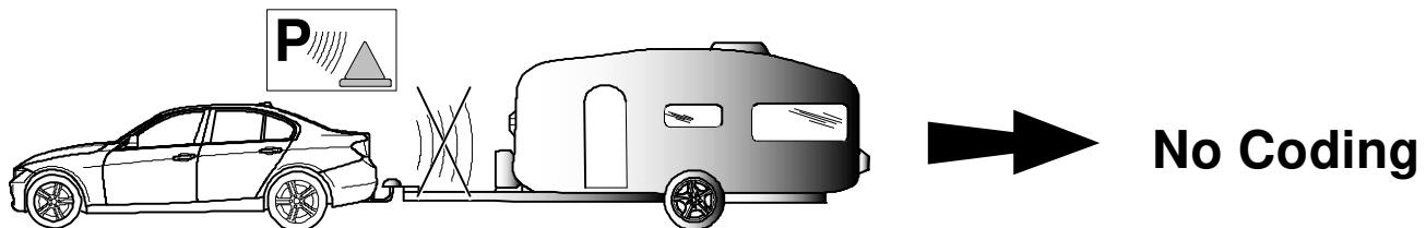
**When PDC doesn't shut off automatically after installation then code vehicle with ISTA/P.**
